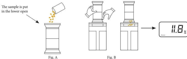
4. Install the filling tube on the instrument transducer port, use one hand to hold the filling tube, and with the other hand, gently press the switch of the material door (as shown in Fig. B), so all samples are dropped into the transducer evenly. Do not press any buttons, the instrument will automatically start, and the moisture value will be presented after the radix point flashes several times:
